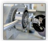
Single-hand locking Simple cutter hub replacement
