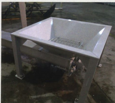
Tramoggia mt. 1x1 con coclea di carico forzato Floor mounted loading hopper mt.1x1 with forced loading screw Grande trémie de charge mt. 1x1 avec vis de charge forcé
